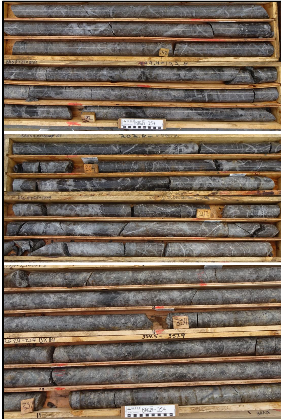
Figure 4. Photos from BRG24-254. Top: strong veining within Berg Stock porphyry with sub-angular clasts of dark biotite altered andesite. Middle: zone of higher grade hypogene copper mineralization with dark biotite altered andesite and lighter Berg Stock porphyry cut by abundant quartz-chalcopyrite-molybdenite and quartz-molybdenite veins. Bottom: intrusive matrix breccia with angular to sub rounded intrusive and volcanic clasts and strong quartz-molybdenite veining.
