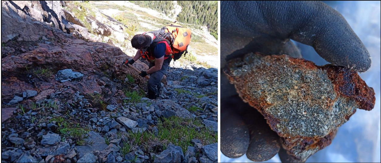
Figure 3. Samples 996352 (4.5 g/t gold, 32.6 g/t silver, and 0.27% copper) and 996353 (8.86 g/t gold, 314 g/t silver, 0.33% copper) from northeast of Bergette. Left: 1 to 2 metre wide rusty alteration zone exposed at sample 996352. Right: Close-up of sample 996353 containing semi-massive pyrite and quartz.
