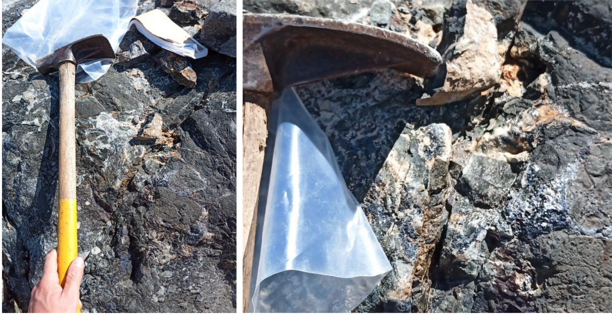
Figure 12. Mineralization north of Whiting Creek. Left: outcrop of quartz veined and siliceous-pyritic volcanic rock sample 996307 (6.25 g/t gold, 35.7 g/t silver). Right: close up of sample 996307 showing quartz veinlets and fine disseminated pyrite and magnetite.
