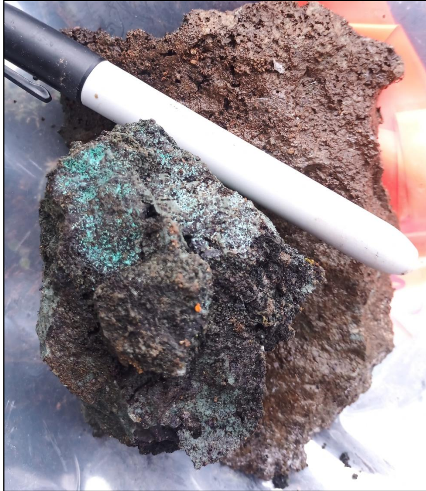
Figure 6. Mineralization at the Sibola Target, sample 997066 (1.19% copper). Altered volcanic rock exposed over 2 metres containing quartz-carbonate veining, iron staining, and malachite.
