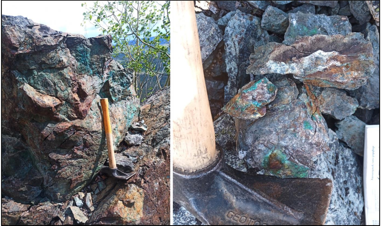
Figure 8. Sample 997128 from north of the Sylvia Target (1.5% copper and 36.1 g/t silver). Left: large green copper stained and mineralized outcrop on ridge top. Right: close up of sample 997128 showing green copper staining and quartz veinlets in silicified volcanic rock containing disseminated chalcopyrite and pyrite.
