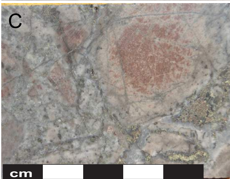
Breccia photos in hole S14-204. A) Rounded matrix supported breccia with both hydrothermal and siliceous intrusive matrix, 369 metres depth. B) Breccia with quartz rich hydrothermal matrix containing sulfides and brown hydrothermal biotite patches, 476 metres depth. C) Close up of intrusive matrix breccia with sulfides pyrrhotite-chalcopyrite-pyrite, 486 metres depth. D) Sulfide rich breccia matrix containing pyrite-pyrrhotite-chalcopyrite-molybdenite, 492 metres depth.
