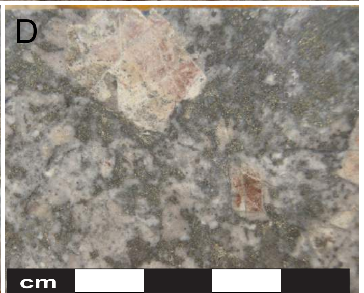
Breccia photos in hole S14-204. A) Rounded matrix supported breccia with both hydrothermal and siliceous intrusive matrix, 369 metres depth. B) Breccia with quartz rich hydrothermal matrix containing sulfides and brown hydrothermal biotite patches, 476 metres depth. C) Close up of intrusive matrix breccia with sulfides pyrrhotite-chalcopyrite-pyrite, 486 metres depth. D) Sulfide rich breccia matrix containing pyrite-pyrrhotite-chalcopyrite-molybdenite, 492 metres depth.
