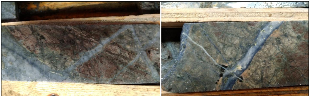
Figure 1. Mineralized drill core from hole S20-220. Left: moderate biotite hornfels cut by stockwork quartz-chalcopyrite-molybdenite veins. Right: molybdenite rich quartz veins with bleached sericite altered halos cutting maroon biotite hornfels.
