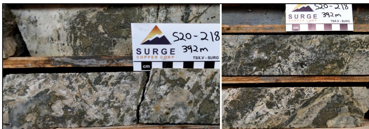
Figure 3. Core from Hole S20-218 around 392 metres depth. Pyrite rich veins and breccias associated with quartz, white clay, and containing low-grade gold mineralization.
